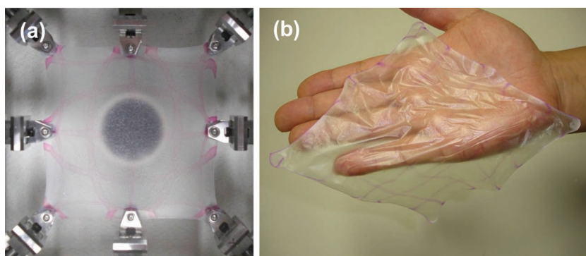
Figure 2. The biaxial drawing machine developed in this study (a) and a biaxially melt-drawn UHMW-PE membrane (b). Drawing was performed at 150\ ^\circ\text{C} . Drawing stresses along both horizontal and vertical directions were recorded by load cells. Eight chucks were designed to grip the sample membrane with air compression, effectively preventing slipping due to the thinning membrane. The thickness of the resultant 8 \times 8 membrane was approximate 1\ \mu\text{m} in (b).
